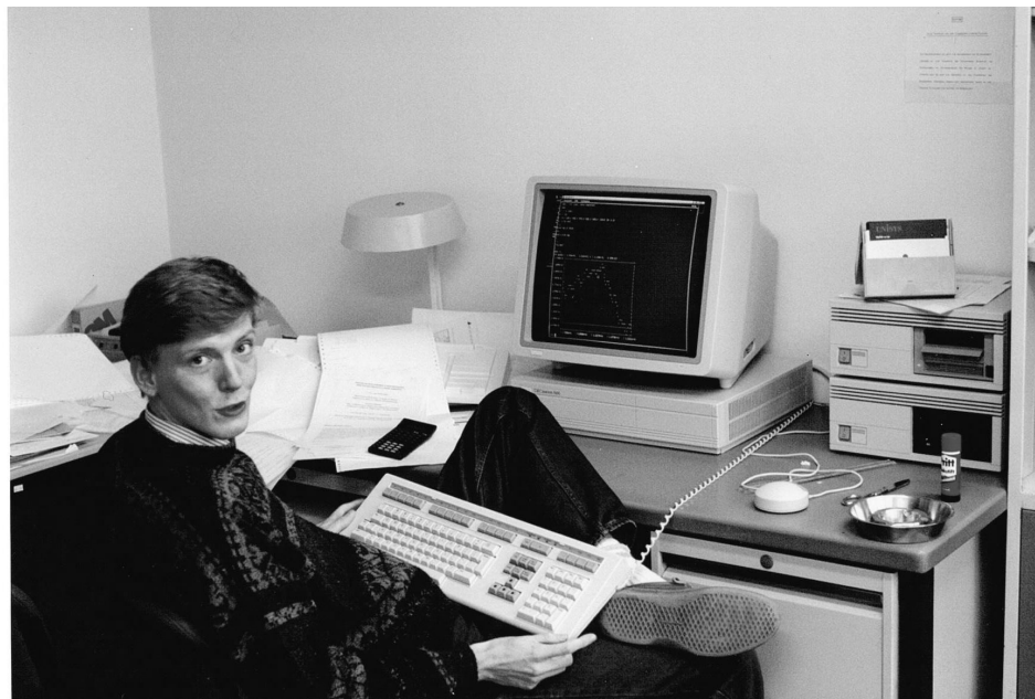
Figure 2.3: Computer simulation in action around 1990. This DECStation 3100 had a 16 MHz RISC processor and 8 MB RAM; it reached circa 2 MFlops. To its right are a tape streamer and a 330 MB disk drive. At the time these DECStations ranked among the fastest UNIX workstations. The one in the photo ran many of the simulations in the original thesis, but also functioned as a terminal for front-ends to the CONVEX or the CRAY. The black-and-white display shows a wildly fluctuating correlation function, obviously to the surprise of the author.
